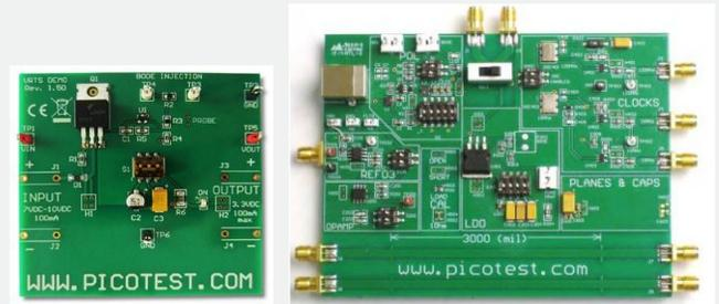
These demonstration boards are self-contained and designed to support a wide range of typical distributed power system measurements including Bode plots and PSRR. Input power is provided via a USB port.
